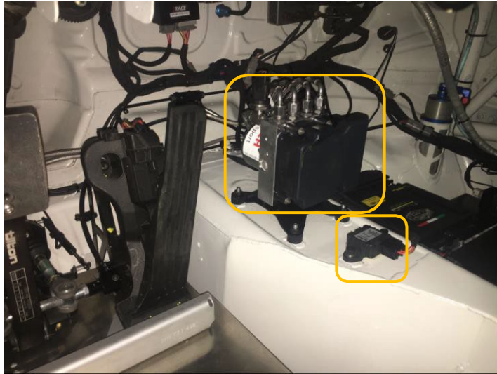
View of the ABS unit and accelerometer in location
