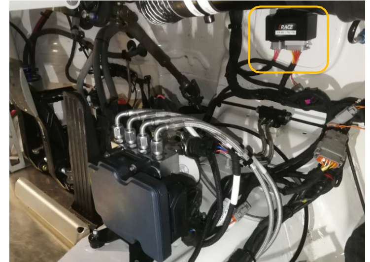
View of the PWB (power box unit) in location Install the PWB using hook and loop tape (3M)
