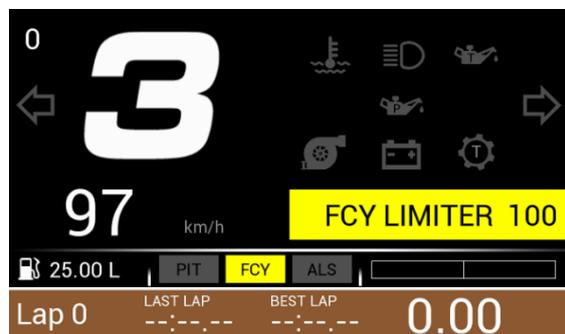
If the car speed is higher than the target limiter speed, check the tyre circumference selected on the ECU clx file (2100 mm as default) that should match with the size of the tires used on the car.
