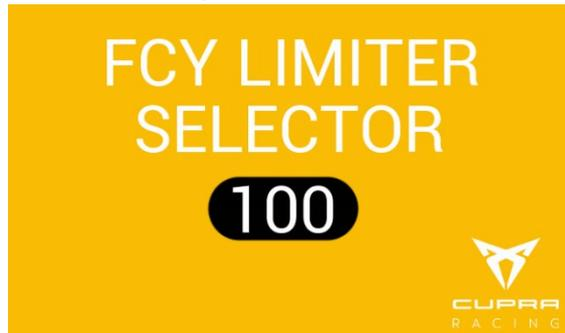
At the Race page, a new flag will be shown, where the driver can see when the limiter is active and the target speed limiter that is selected. With this layout, the driver can quickly check if the car speed is higher than the selected one.
