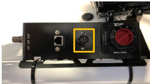
3. Select the rotary switch on the Laptop Tool at the second position (GATEWAY) and check the Boot switch is not activated.
