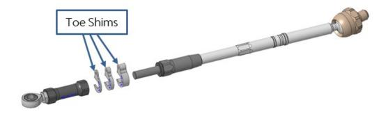
Additional fine tuning can be made by turning the outer ball joint.
