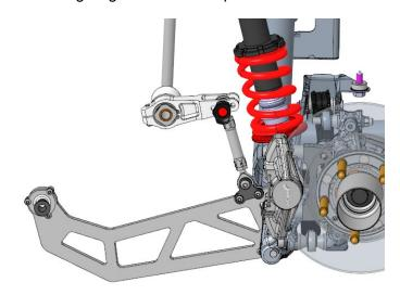
In the same way as on the front axle, each lever has been designed with three holes in order to be able to change the stiffness in smaller steps. The fixation to the drop link can be made with the quick-release pin (car delivery) for quick changes or a standard bolt can replace it.
