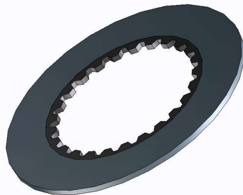
Revised Specification (MOLY) Part No. TPT-213-8B Thickness = 1.95-2.0mm
