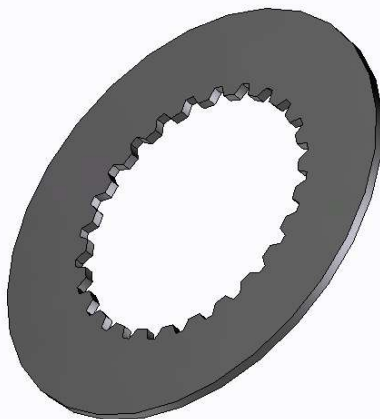
Previous specification (PARCO) Part No. TPT-213-8 Thickness = 1.6-1.7mm
