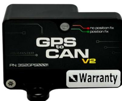
To solve this issue, customers who has this GPS to CAN V2 module (Leon VZ) must upgrade the FW version using the Software **LightClientSetup\_2\_0.exe** and **gps2\_fw4\_0.bin** file. SW and FW files are available on the VW Group Motorsport online platform download area at the path "PROJECTS & SOFTWARE / SW\_PROJECTS\_2024 / GPS FW / CUPRA LEON VZ".
